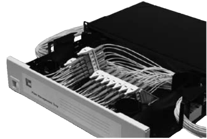
Sliding Adapter Pack (shown in access position)
